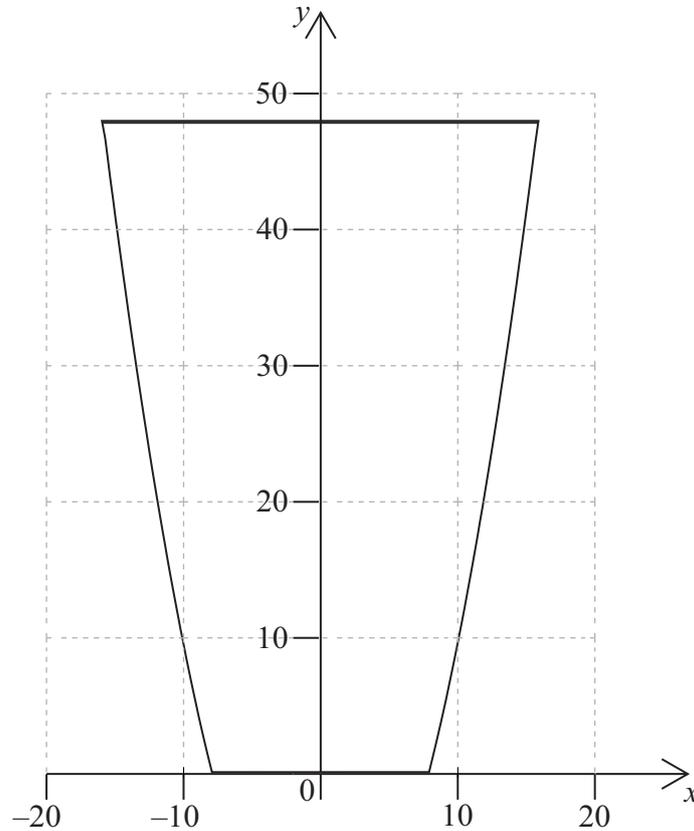
The curved sides of the cross-section are given by the equation  $y = 0.25x^2 - 16$ . The horizontal cross-sections are circular. The depth of the container is 48 cm.
